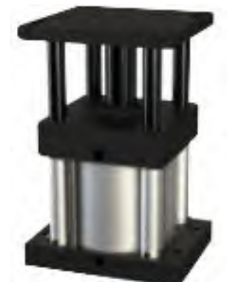
Lifter 4 Post. Ex: 5" bore, 4" stroke, main rod 1.75" dia and the 4 post at 1" dia. The post are guarded by thin wall tubing.
