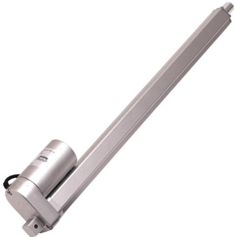
Premium High Force Linear Actuators offer an astounding 400 lbs of force in the same compact and versatile design as the Classic Actuator. With an IP rating of 66 and strokes available from 2 - 30 inches, this actuator is suitable for almost any environment. The high grade aluminum housing resists corrosion and provides you with maximum life and value.
